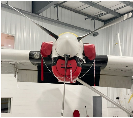
DeHavilland DH-6 Intake Plugs, Exhaust Covers Prop Tie-Down, Various Models (secures with a hook to engine nacelle)
