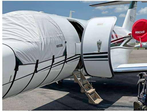
Cessna Citationjet 525C, CJ-4 Engine Inlet Covers & Exhaust Plugs
