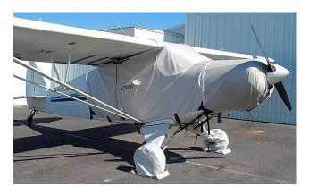
Piper PA-12 Extended Canopy, Engine & Landing Gear Covers
