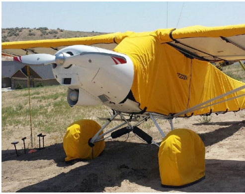
Piper PA-18 Super Cub Extended Canopy Cover, Wing & Tire Covers Cub Crafters Tire Covers, tricycle gear, test fit covers
