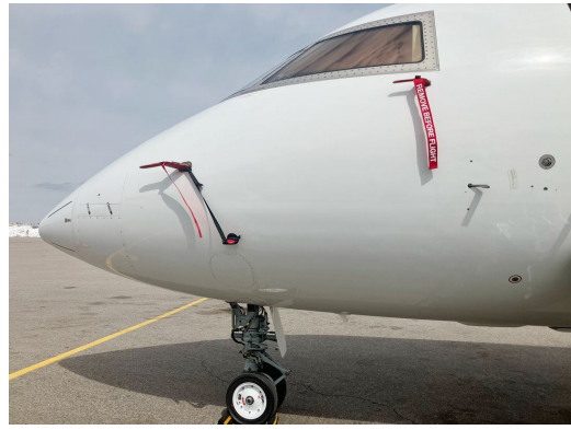
Challenger 650 Pitot & Ice Detector Covers
