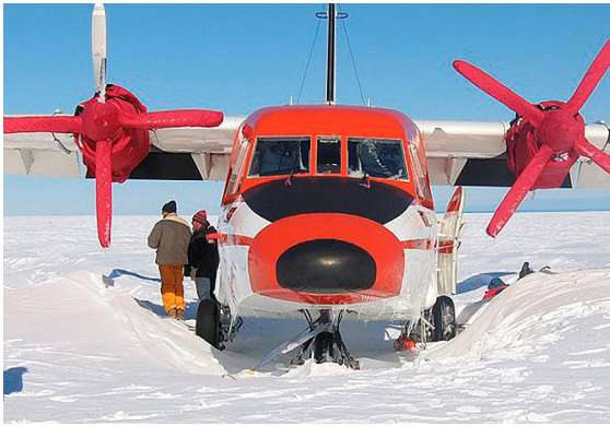
Casa 212 Insulated Engine & Propellor/Spinner Covers
