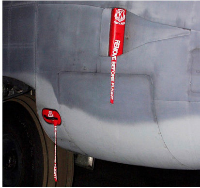
C-130 Heat Exchanger & Exhaust Plugs
