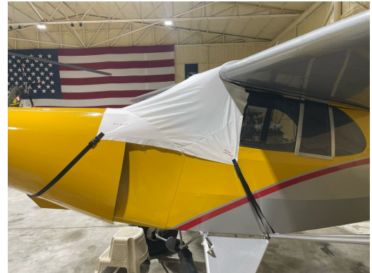
Piper J5A Windshield/Skylight Cover, test fit
