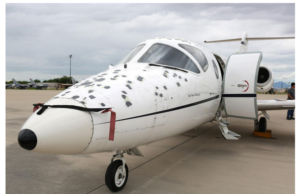
Raytheon Beechjet Hail Damage, and Pitot Covers
