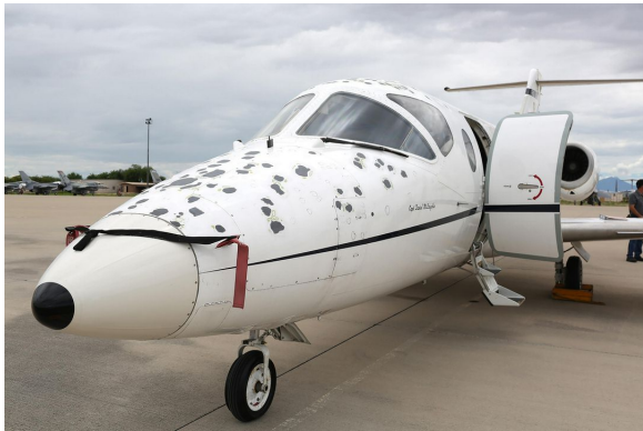
Raytheon Beechjet Hail Damage, and Pitot Covers
