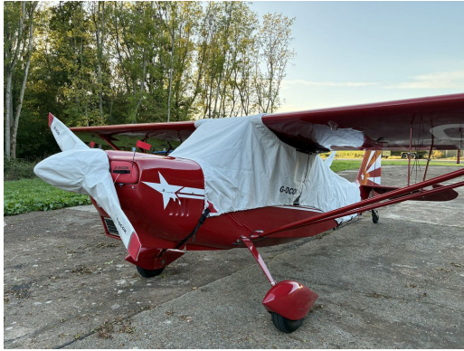
Super Decathlon Canopy Cover, Over-Top with Ext. to Tail, Prop Cover, Engine Plugs.
