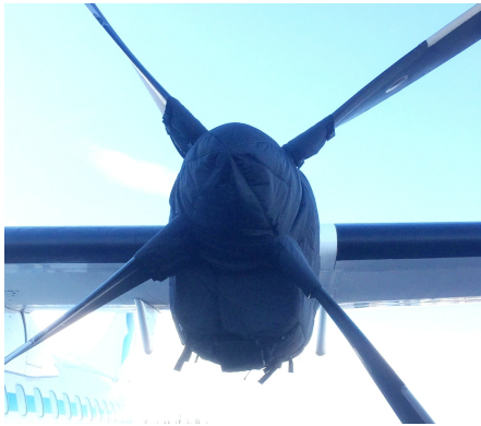
ATR-72-202 Insulated Engine & Prop Hub Covers
