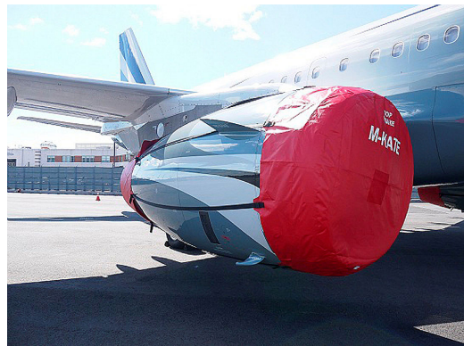
Airbus A319 Intake/Exhaust Covers set, IAE V2500
