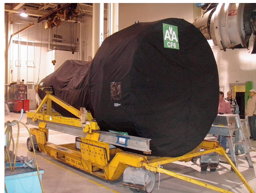
GE CF6 Series Off-Link Engine Shipper Cover, w/ Exhaust Cone, Fully enclosed
