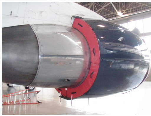
Boeing 767 Exhaust Plugs Ship Set, incl. Fan Thrust Reverser and Exhaust Plugs P/N: B767-200
