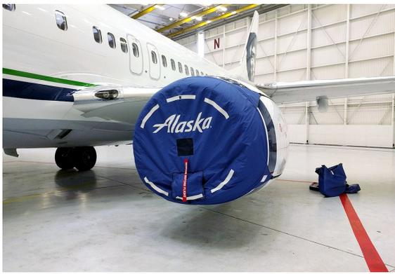
Boeing 737 Intake Cover w/ Heater Attachment
