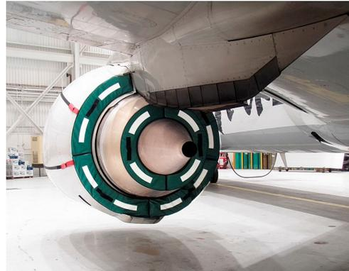
Boeing 737 CFM-56 -400 Exhaust Plug with reflective imprint
