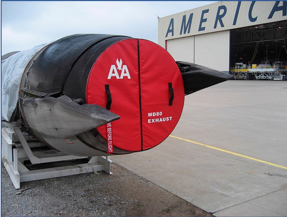
MD80 JT8D Exhaust Plug, Folding Type
