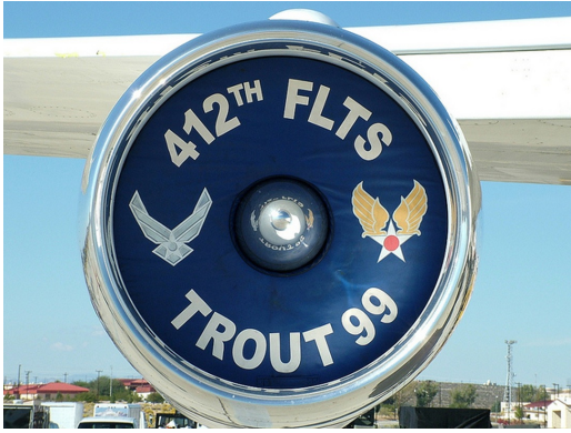
Boeing KC-135 Engine Inlet Plug, TF-33
