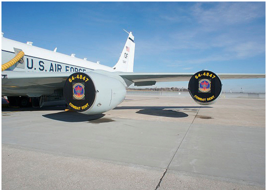
KC-135 “Tambourine” style, Double Fold Intake Covers with artwork KC-135 Intake Covers for the 55th ARW, Offutt AFB
