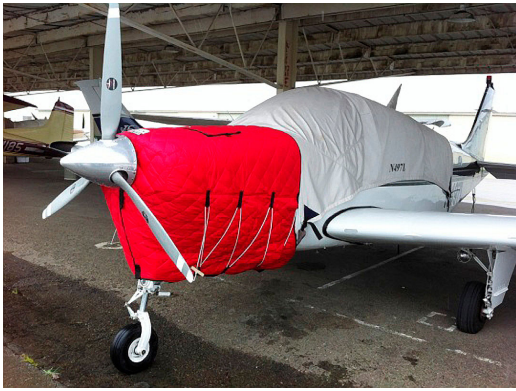
Beech Bonanza Insulated Engine Cover, fully enclosed
