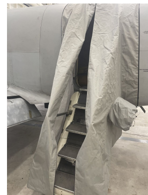
King Air Airstair Door Cover
