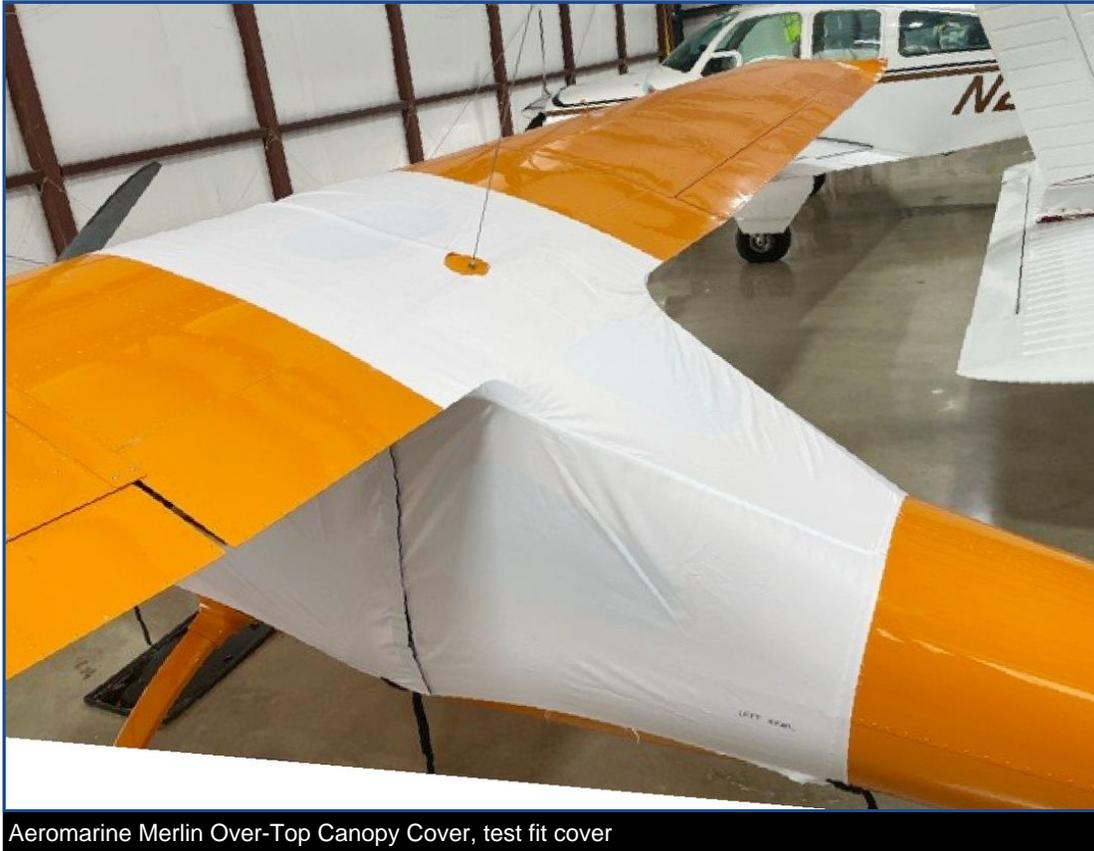
Aeromarine Merlin Over-Top Canopy Cover, test fit cover
