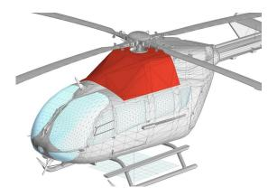
Barrier Inlet Filter Cover, 3D Rendering
