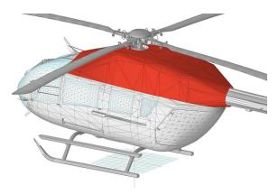
Intake/Exhaust Engine Area Cover, 3D Rendering
