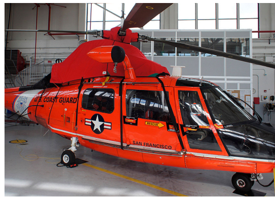
MH-65C Engine Area Cover, Swash Plate Aperture, Rotor Hub cover set, P/N: A365-210
