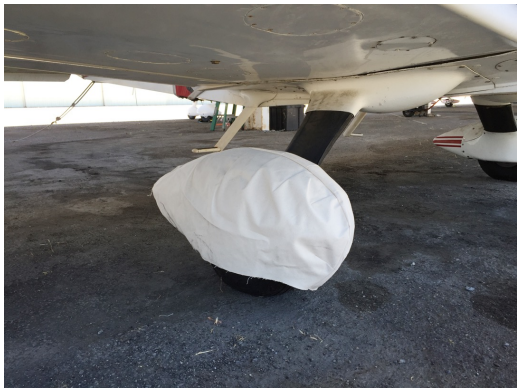
Grumman AA5 Main Wheelpant Cover, test fit
