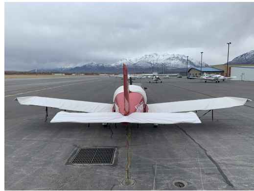
Grumman AA-1 Wing & Horizontal Stabilizer Covers
