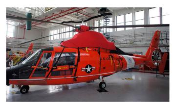
MH-65C Rotor Hub, Swash Plate Aperture, Engine Area Cover set, P/N: A365-210
