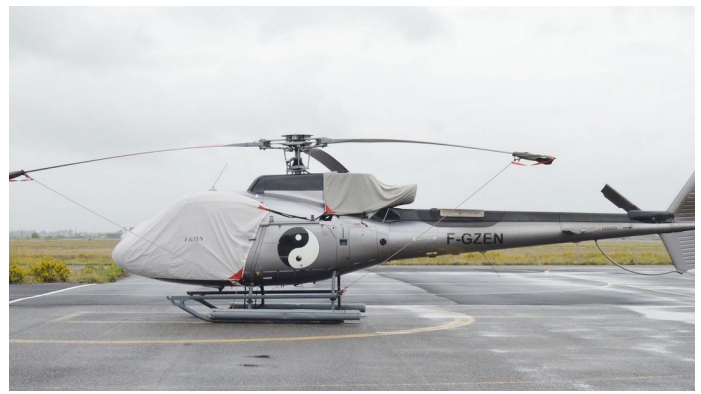
Airbus Helicopter AS350 Bubble Cover & Intake/Exhaust Cover
