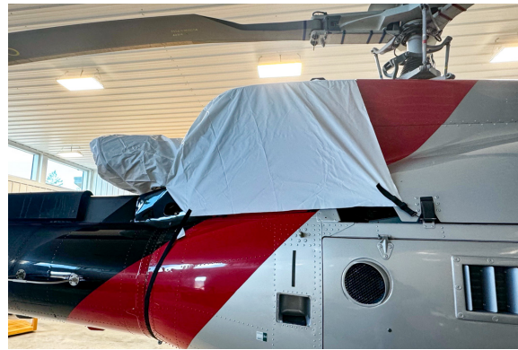
Airbus Helicopter AS350-B3 Intake/Exhaust Cover, test fit cover
