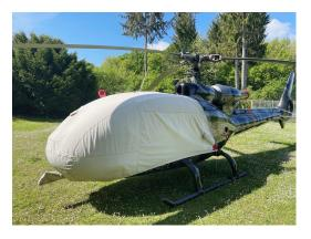
Gazelle Bubble, Abbr. Engine, Rotor Hub, Blades & Fenstron Covers (Illustration)
