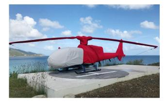
Aerospatiale Gazelle AS341 Bubble, Rotor Mast, Blade, Engine & Tailboom Covers (some are test fit covers)
