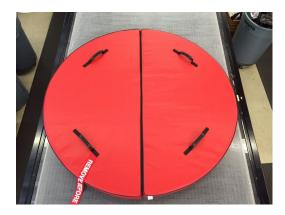
Boeing 737 Max Intake Plug, folding type
