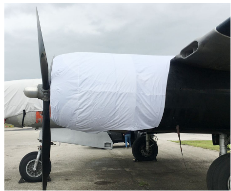
Douglas A-26 Engine Cover, test fit cover
