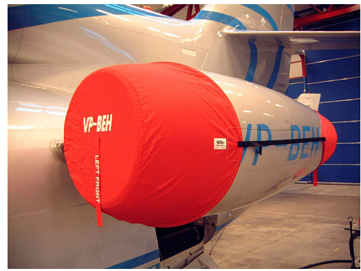
Falcon 900 Engine Covers, outboard & inboard strap detail
