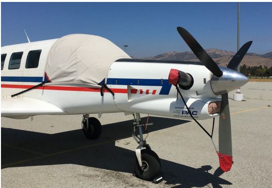
750XL Combination Insulated Engine Cover/Cockpit Cover Pacific Aerospace 750XL Cockpit Cover, Prop Tie/Exhaust Covers
