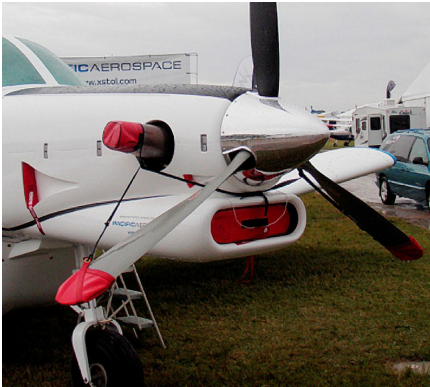
750XL Engine Inlet Plugs & Prop Tie/Exhaust Covers
