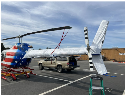
Bell 505 Tailboom & Stabilizer Covers, test fit cover
