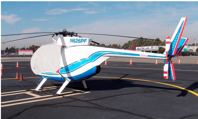
MD500C Bubble Cover with Wire Strike detail
