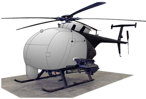
MH-6J Bubble, Flir & Doghouse Covers (illustration)
