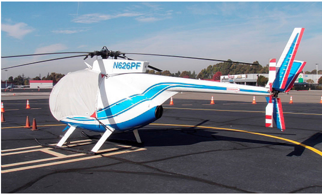
MD500C Bubble Cover with Wire Strike detail
