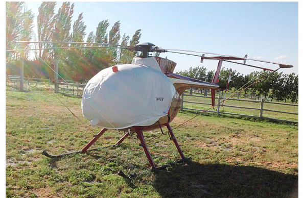
MD500D Bubble Cover with Intake Add-On
