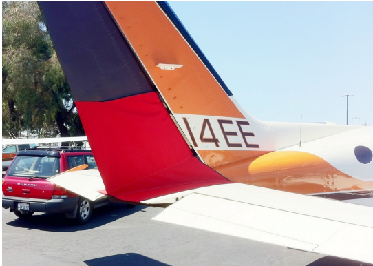
Cessna 414 Rudder Openings Cover (bird barrier)
