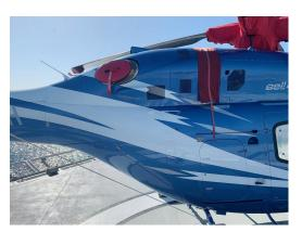
Bell 429 Exhaust Plug, Rotor Mast Cover
