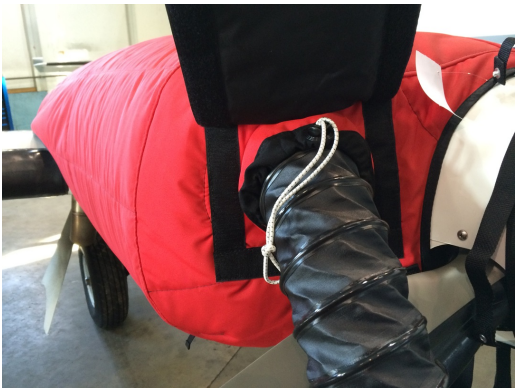
Cessna 402 Insulated Engine Cover with Heater
