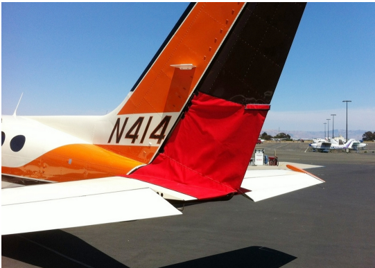
Cessna 414 Rudder Openings Cover (bird barrier)
