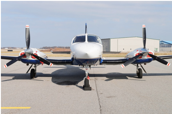
Cessna 421C Engine Inlet Plugs
