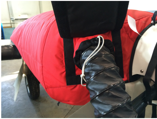
Cessna 402 Insulated Engine Cover with Heater
