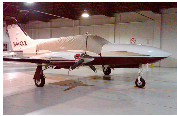
Cessna 414 Canopy Cover and Engine Inlet Plugs
