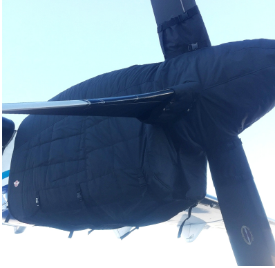
ATR-72-202 Insulated Engine & Prop Hub Covers
