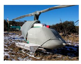
JetRanger Bubble, Engine, Rotor Hub & Blade Covers (& Tie-Downs)
