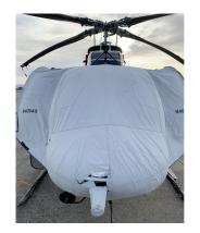
Bell 407 Abbreviated Bubble Cover, secures to doors, test fit cover
