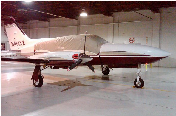
Cessna 414 Canopy Cover and Engine Inlet Plugs
