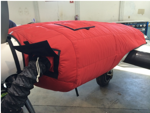
Cessna 402 Insulated Engine Cover with Heater
