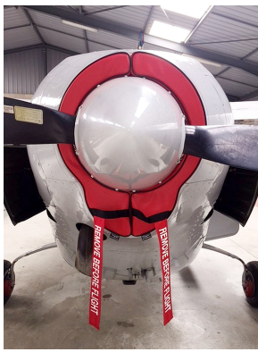
Cessna 337 Skymaster Aft Engine Outlet Plugs
