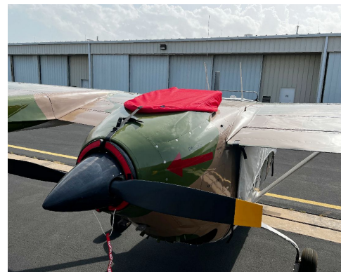
Cessna 337 Skymaster Aft Engine Inlet Cover & Plugs
