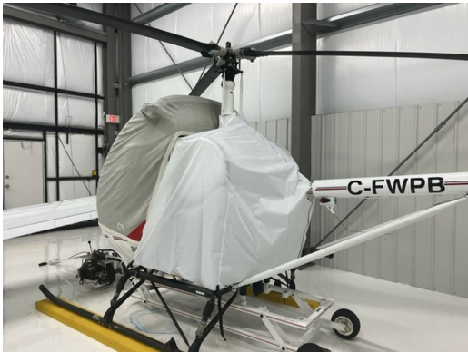
Schweizer 300C Engine Cover, test fit cover
