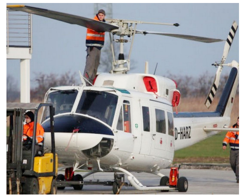
Bell 212 Main and Oil Cooler Intake Plugs
