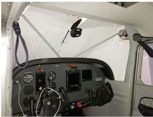
Cessna 180 Skywagon Windshield Heatshield, (W/ Compass)
