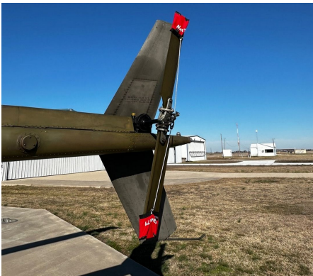
Bell 206B Jetranger Tail Rotor Tie-Downs
