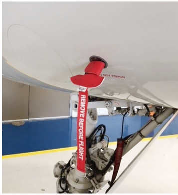
Grumman Gulfstream G-V Rosemont/TAT Cover Falcon Jet 2000 Pitot Covers, Aoa's, Tat Cover Set, Heat Resistant Type
