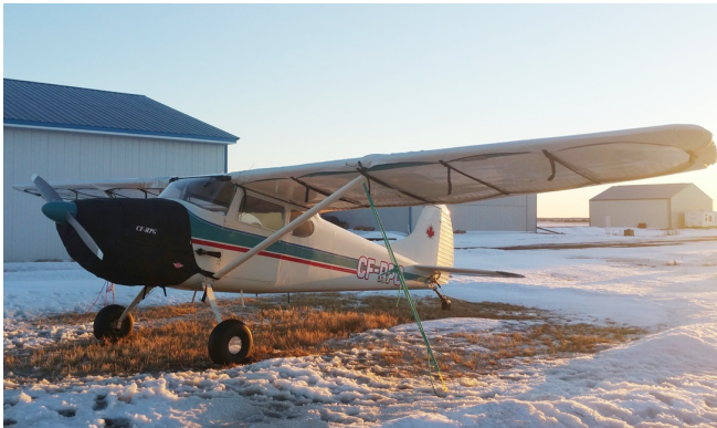
Cessna 170 Insulated Engine Cover, Wing Covers
